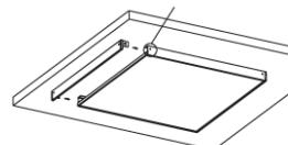
2. Fix the aluminum frame with screws
