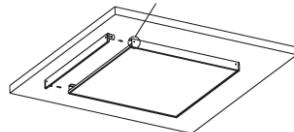
2. Fix the aluminum frame with screws
